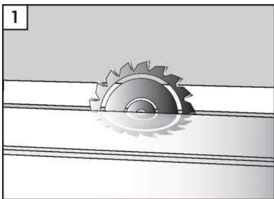
1. When cutting, a buttress gear saw should be used.
